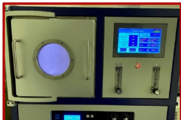
Plasma Treatment to enhance adhesion with electrode
