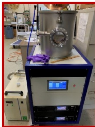
Magnetron Sputter Coater with turbo pump for Cu, Cr, Ti, Au, Ag, Al, Pt Two targets φ 300 mm SS chamber
